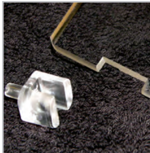
Clips are inserted into notches cut into the acrylic to hold dividers secure
